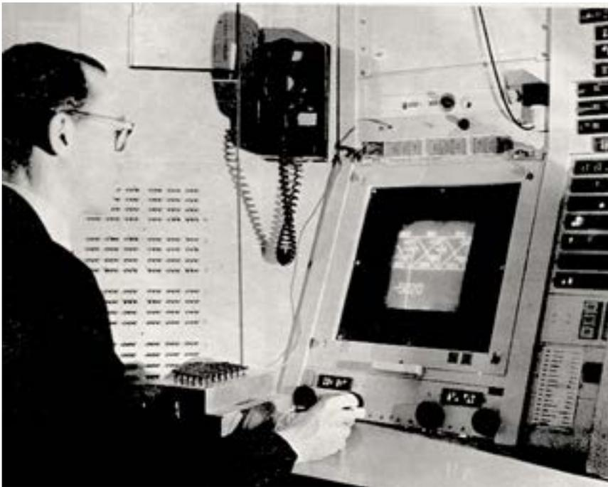
Figure 5. Sutherland operating Sketchpad on the TX-2 computer at MIT, 1963. (By courtesy of MIT)
