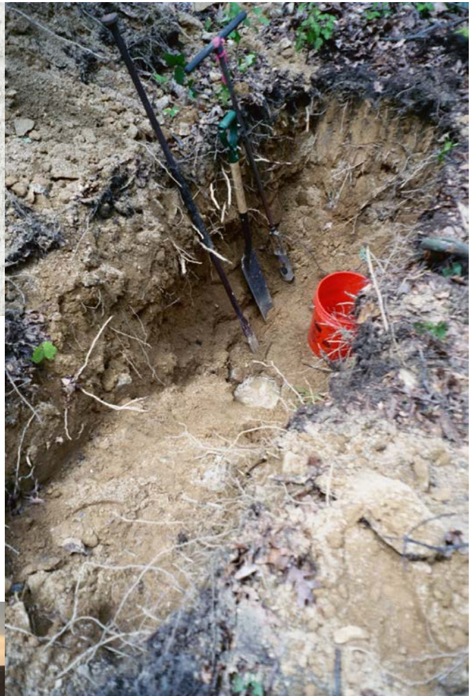
Figure 20. Perk tests, conducted along the East Branch of Brandywine Creek by the author, provided a close reading of the site, integrating the proposed dwelling units with erosion and sediment controls and accelerating the approvals process. Moreover, the deep memory remained of the scent of freshly cut sassafras roots, several feet below the cool soil on a hot summer day. (Photo by author)
